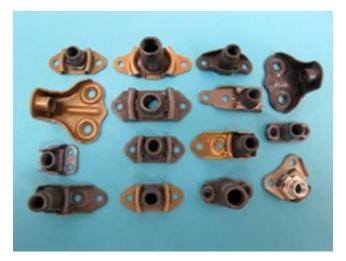
Pictured are some of the various surplus Boeing nut plates we have in stock. They come in 1 lug, 2 lug, floating, right angle, and corner or side by side floating configurations.
